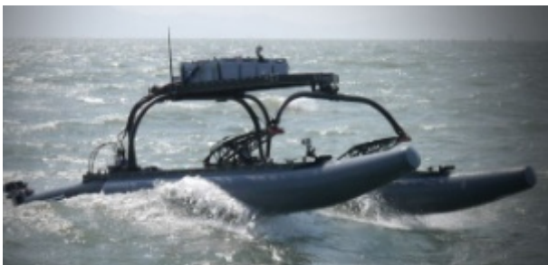
Fig.1 16 WAM-V USV, with the length of 4 m and the weight of 100 kg without payload.
